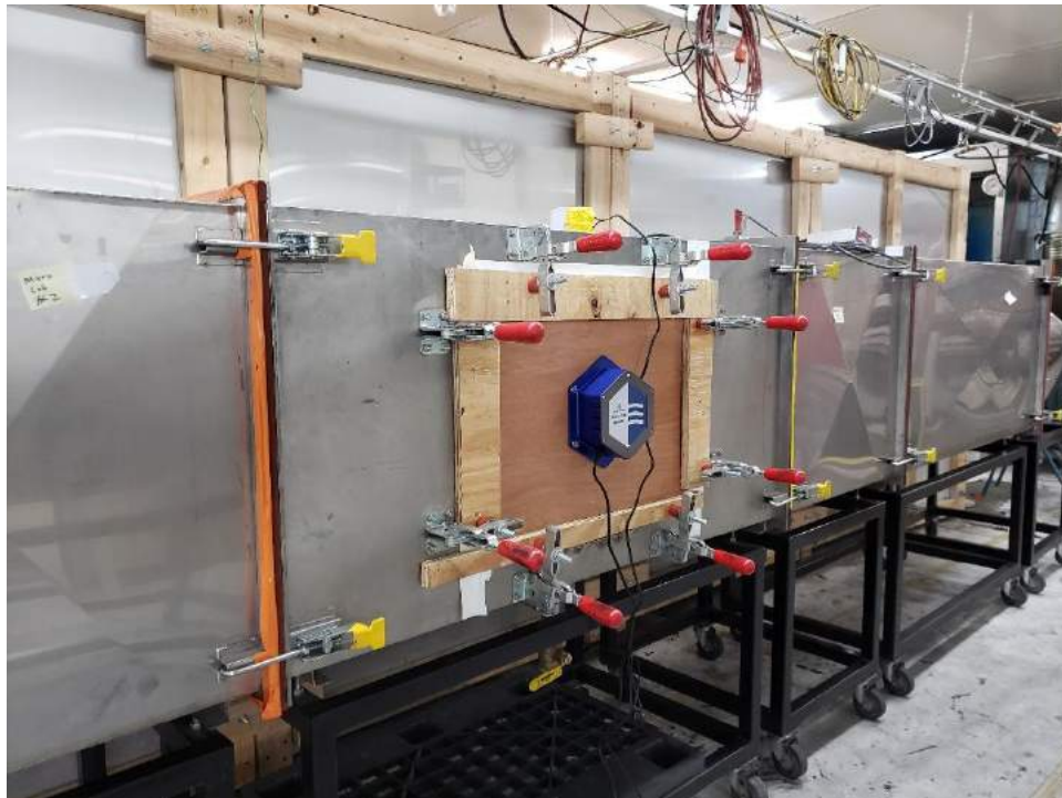
Figure 3. Dust Free Active Air Cleaner mounted in 24"x24" test duct
