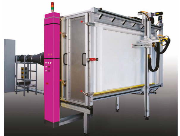
Photo : Essai de scanning - EN1822-4
