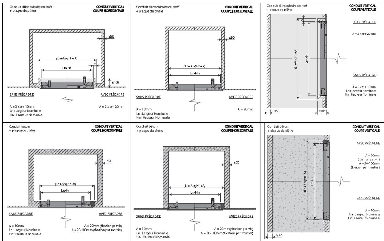
**7.4. MISE EN ŒUVRE D'UN MUR DEVANT LE MANCHON OU LE CONDUIT DES VOILETS**
