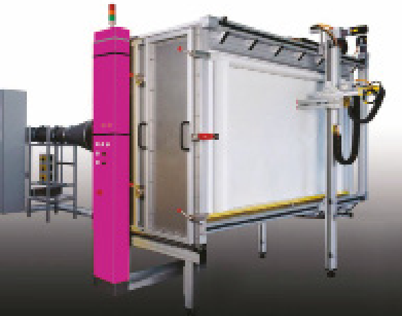
Photo : Essai de scanning - EN1822-4
